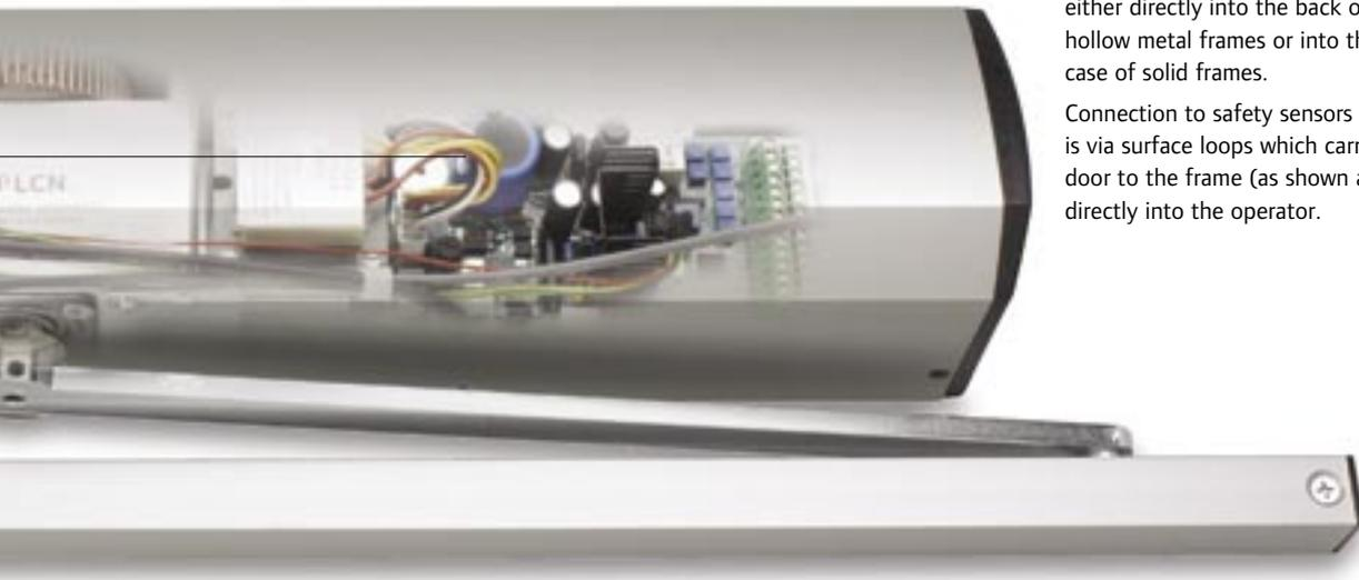
Mains power to the low energy operator can be fed either directly into the back of the unit in the case of hollow metal frames or into the end of the unit in the case of solid frames.
